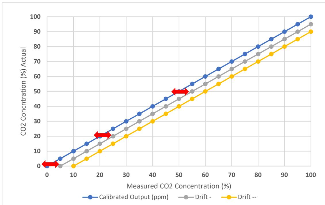
The change in reference level of the sensor can be cancelled out using a process known as zero-setting. This resets the sensor to a defined concentration level.
