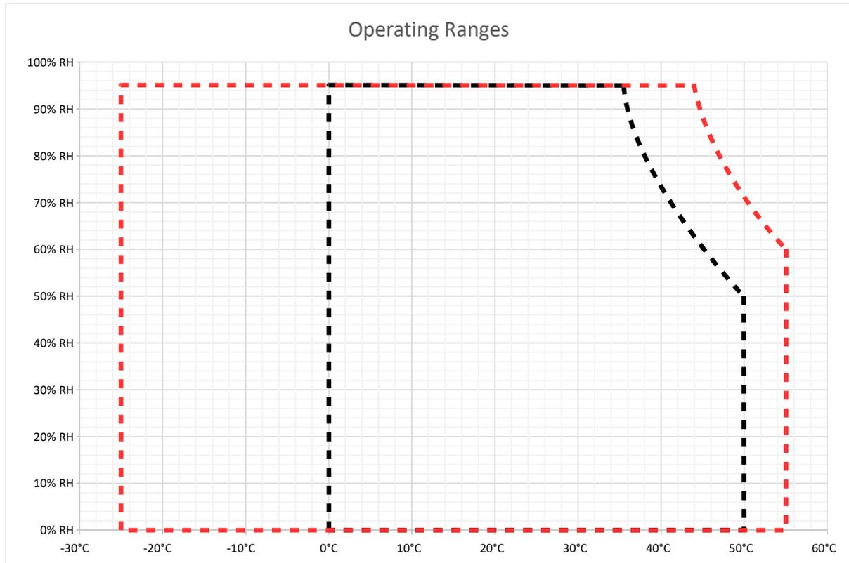
However, using the above formula, at 95% relative humidity, there is only a 1°C difference between the ambient temperature and the dew point temperature.
