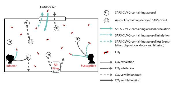
Figure 1: Illustration of mechanisms for increasing and decreasing CO<sub>2</sub> levels and virus transmission in a ventilated indoor environment. The grey arrows denote movement of virus particles, and the blue arrows illustrate CO<sub>2</sub>. The mechanisms for decreasing virus particles are by natural decay and removal by ventilation or filtration. [1]
