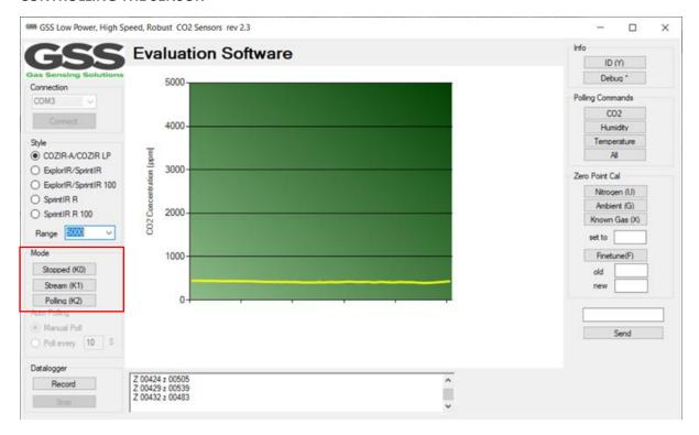
The software interface replicates the UART controls of the sensor. For full details of the functions, refer to the product data sheet. After power is applied, the sensor will automatically start to take  $CO_2$  measurements using the Mode 1 default settings, where the sensor is pre-programmed to send  $CO_2$  measurement data. This mode is labelled as 'Stream (K1)' mode.
