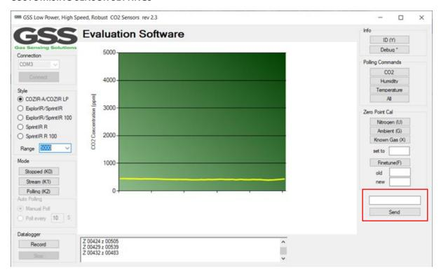
The evaluation kit software allows the user to fully customise the settings of the sensor. Refer to the sensor data sheet for a full command and control description. All UART commands and functions of the sensor can be manually set by writing in the blank box with the correct syntax. To send an UART command or data to the sensor, write in the blank box and click the 'SEND' button.
