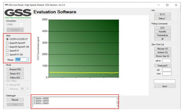
Select the correct sensor type and the full-scale range ( $CO_2$  ppm) of the sensor. The sensor should automatically start to take  $CO_2$  measurements after 1-2 seconds. These measurements are shown graphically in the middle of the screen, and in the dialogue box (red) at the bottom. The dialogue box contains sensor serial data output ('Z' data). The  $CO_2$  'Z' value needs to be scaled to calculate the ppm value.
