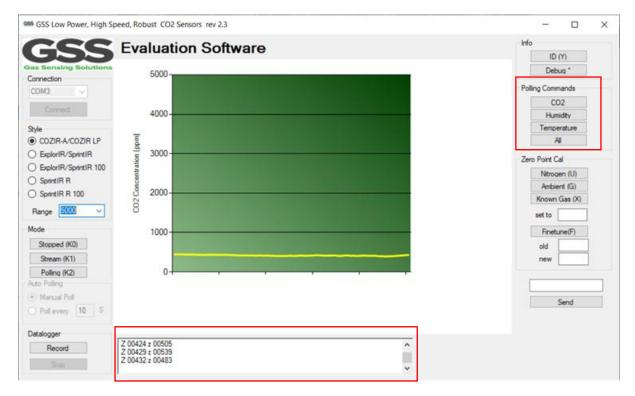
Depending on the sensor type, various parameters can be output as a single string of data in the dialogue box. If a temperature or humidity sensor is fitted, the dialogue box will show the relevant data fields depending on user requirements.
