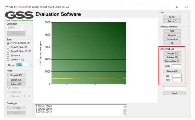
There are a several methods available to the user to set the zero point of the sensor. In all cases, the best zero is obtained when the gas concentration is stable, and the sensor is at a stabilised temperature. Note the zero-point settings are not cumulative and only the latest zero-point setting is effective. For example, there is no benefit in zeroing in nitrogen, and then zeroing in a calibration gas. The sensor will store only the latest zero point.
