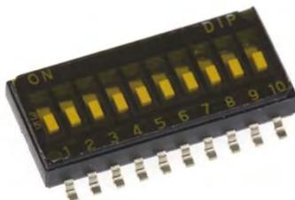
**Figure 4: DIP Switches (S5, shown in OFF position)**
