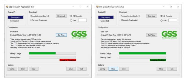
The evaluation platform can now be disconnected from the USB cable and will record data autonomously. The LED on the EvaluatIR-A will flash briefly at each reading point. Note that if the measurement interval is long, this will happen infrequently.
