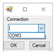
Select the correct COM port and click on the 'Connect' button. The software application will now show the unit is connected, the battery level and the memory status.
