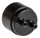
The SprintIR<sup>®</sup>-R is based on GSS proprietary solid-state non-dispersive infra-red (NDIR) LED technology, where the sensor measures concentration levels by analysing the amount of light absorbed by the CO2 gas. The ability to measure CO2 gas levels at unprecedented rates is due to a combination of GSS solid date detection technology with its inherent high response rate, and special optical design techniques.
