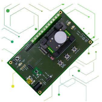
When using the Sensor Evaluation Board, a GSS CO<sub>2</sub> sensor can be separately powered and all features brought out at the board edge for customer evaluation. The SEB can also be used to set up and zero a sensor remotely.
