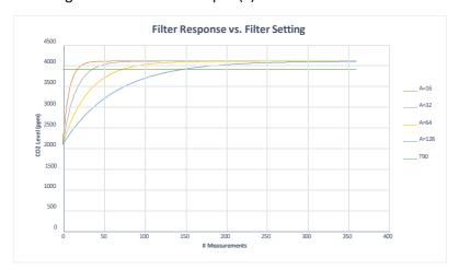
The graph above shows the effect of the filter on response times. Increasing the filter setting increases the measurement output response time.
